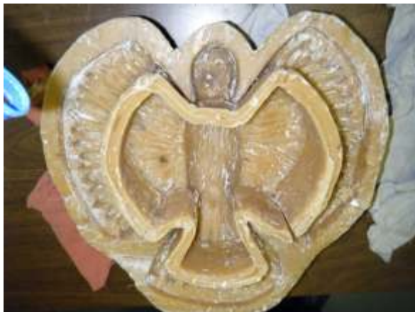
Wax prepared for hot-pour bronze mould
